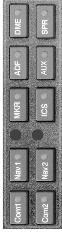
heard, the **Com 1** and **Com 2** push-buttons are of the momentary type and do not remain in when selected. This is also part of the "auto" function. You will always hear the audio from the transceiver that is selected for transmit by the rotary mic selector switch.
